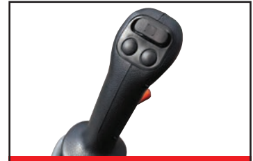
Hydraulic Pilot Controls
