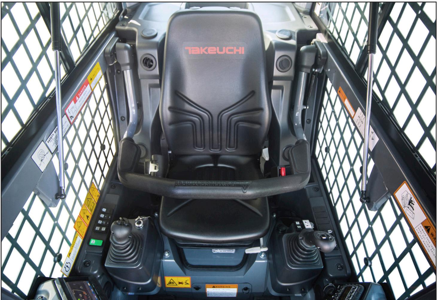
Spacious operator's platform with easy to reach controls and switches.
