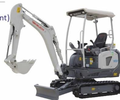
TB20e lithium-ion battery-powered compact excavator
