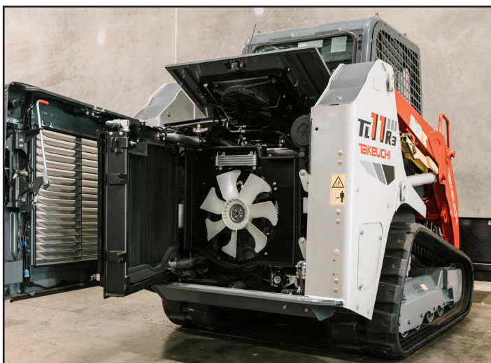
Swing-Out Cooling Module for Easy Cleaning
